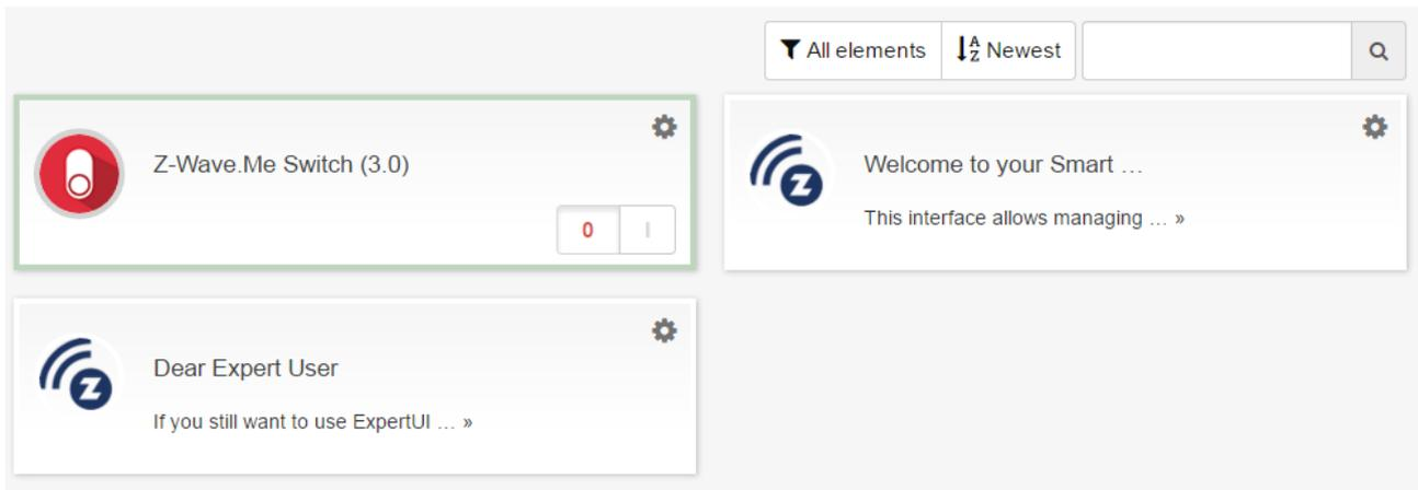
To adjust Element configuration, click “Settings” icon at the top right corner of the UI block corresponding to the Element. This will open the “Element Configuration” screen.
